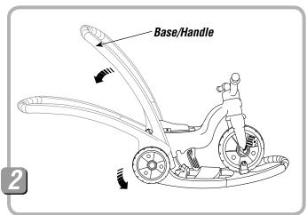
• Rotate the base/handle down, under the trike, to the ride-on rocker position.
